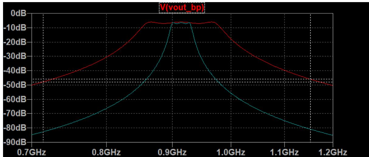
Simulation of the 3<sup>rd</sup> order Chebyshev filter with a Q of 8 (red) and with a Q of 30 (cyan) to highlight our RF BW. You see the margin that is kept to account for component mismatch. Again an implementation of a filter with a Q of 30 is not feasible with LC components due to the large ratio required (>2000) and the component spread that shifts the curves laterally. Even with a Q of 8, the image band attenuation is >45dB (cursors centered at 715 and 1115 MHz).
