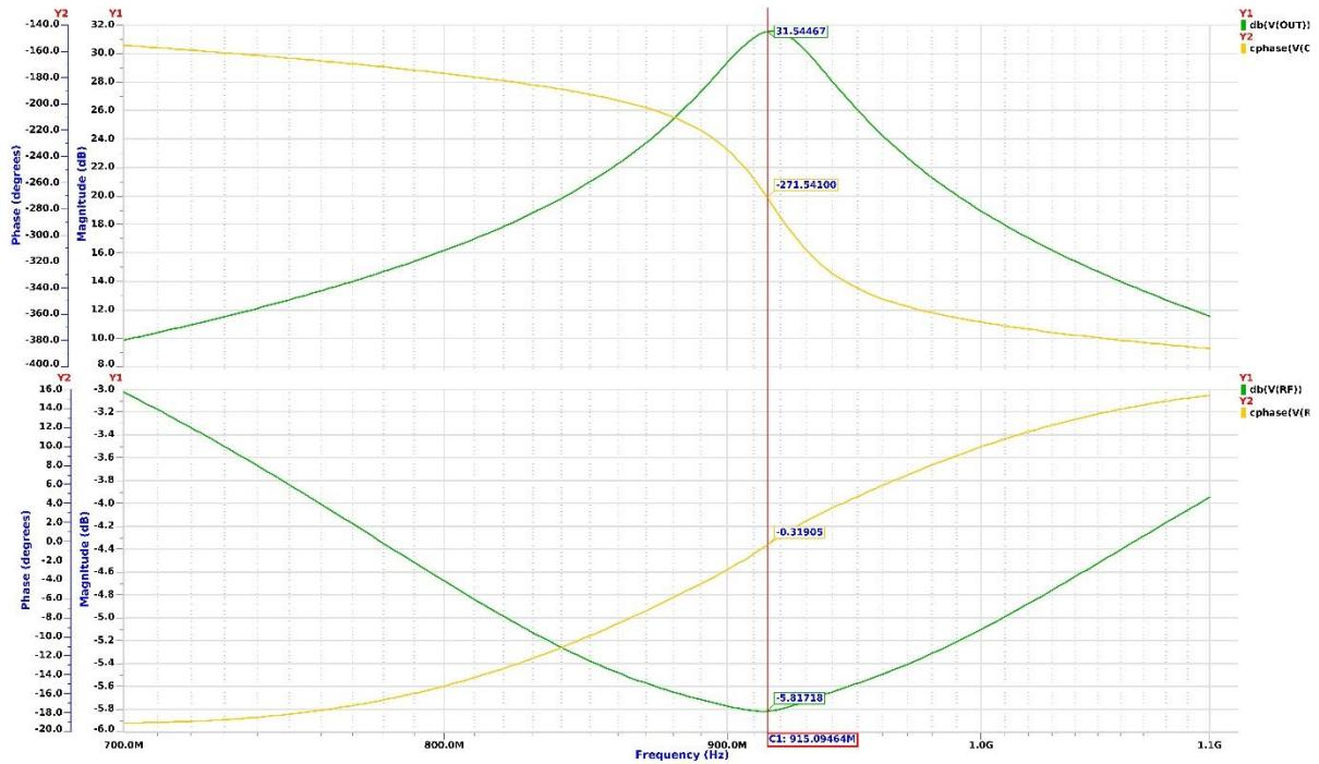
The circuit with  $R3=20\text{ k}\Omega$  is now loaded with a  $75\text{ }\Omega$  resistor and impedance matched so that the loaded  $R$  is still  $10\text{ k}\Omega$ . The top above plot shows the  $V3$  node output magnitude (31.5dB of gain) and phase. The bottom one shows that the input node is impedance matched (6dB attenuation, 0 phase near 915 MHz).
