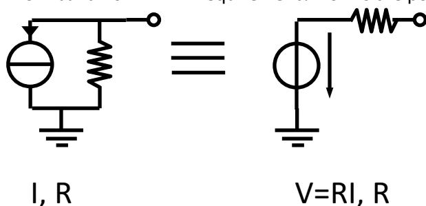
Our LNA output is a current source (MOS) with a loading resistor. It is equivalent to a voltage source  $RI$  with a series resistor  $R$ . We may thus match it so that the filter sees  $75 \Omega$  with an LC L network.
