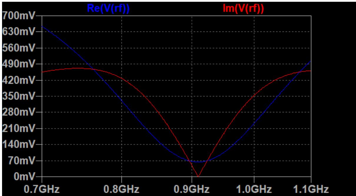
Plot of the real and imaginary part of node 1 (LNA input, matched to  $50\ \Omega$ ). We should get 0.5V instead of 70mV ! The imaginary part indeed goes to 0 at 915MHz.
