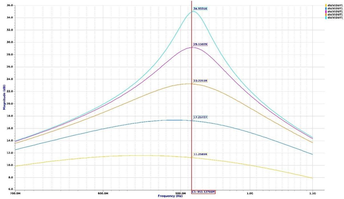
The voltage gain is plotted above for various output resistances (1, 2, 4, 8, 16 kΩ). The gain indeed increases by ~6dB each time R3 is doubled. Note that C3 was adapted to center the curves at 915MHz.
