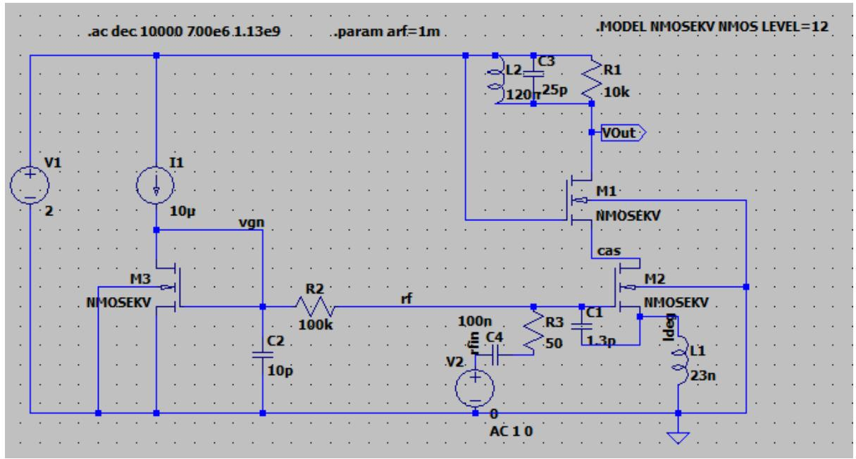
Schematic above with 160uA in M2 (m=16 using same MOS as mixer, cascode identical), note the bulk connections to GND (body effect accounted for). An ideal AC-coupling cap (C4) added to isolate the input source from the LNA DC bias.
