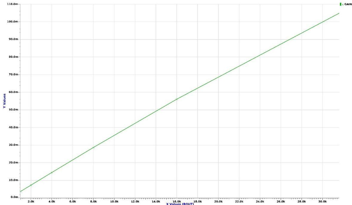
In a transient simulation, the gain is extracted again vs the output resistance and shown in the above plot. Rout=10k corresponds to a Q of 15. With L3/L2=120/23, the voltage gain is expected to reach 39 according to our calculation ( $L3/L2 \cdot Q/2$ ). We read 35, this is much closer. You may notice the saturation of the gain at large Rout (likely due to output conductance and/or frequency selectivity and slight resonance offset).
