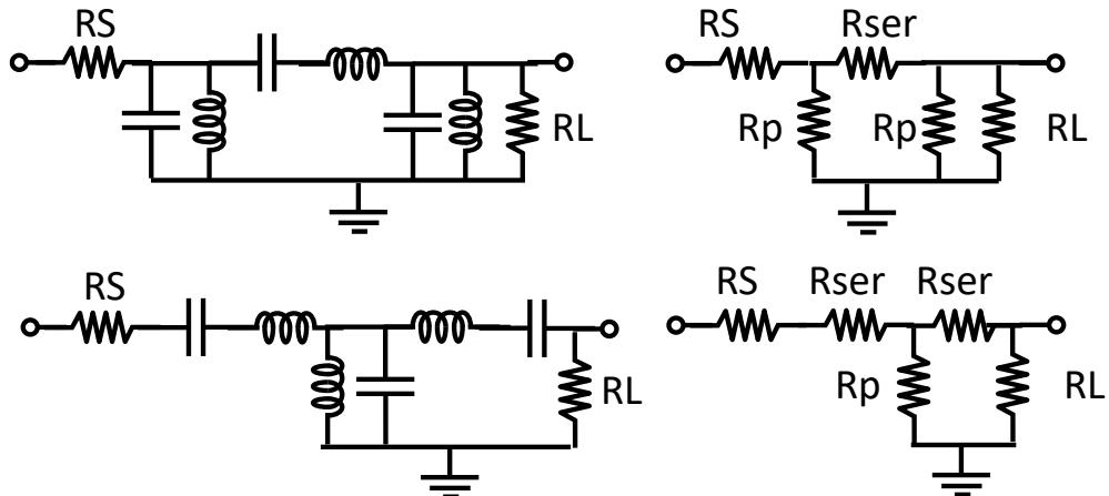
e) select the input/output resistor and Q value so that the filter could be designed with the available components
