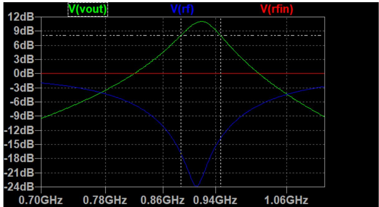
Plot of the LNA gain (11dB). The BW is 61MHz indeed corresponding to a Q of 15. The input voltage should be at -6dB due to input match (it is 18dB lower, factor 8!). This is again a problem of LT spice!
